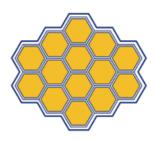
Bundles made from end-fused fibers show no gaps between individual fibers, since the fibers attain a hexagonal shape during the fusing process.
